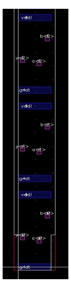
Finally, as with any layout, run DRC, Extract, and LVS. The only difference with this cell is that you will need to check the 'Join Nets With Same Name' box in both the DRC and Extract windows so that the tools know you intend to connect gnd! and vdd! later on. Be sure that you eventually do so before finishing your chip; in our case, we will provide power and ground rings in Lab 4.
