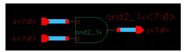
First instantiate an and2\_1x from muddlib11. Choose Edit • Properties • Object... and change the Instance Name to and2\_1x<7:0> to create 8 copies. Create the input pins (a<7:0> and b<:0>) and output pins (y<7:0>). Choose Add • Wire (wide) and draw busses between the pins and the gate. Check and save and ensure you have no errors.
