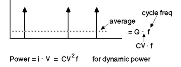
This is a fundamental power that is needed to switch capacitors (without inductors).
