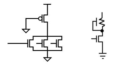
In a 1 $\mu$  technology, the current is 170 $\mu$ A/ $\mu$  of width for the pMOS. This means that the current for a 4:2 device would be around 340 $\mu$ A, and the power would be 1.7mWatts (on average) for the gate. 10K gates --17Watts
