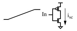
In general the percentage of the total dynamic power due to the short circuit current is much smaller than that used to charge and discharge the capacitive loads. Very slow rise and fall times on the inputs could however make this current significant, and must be considered for gates at the end of long wires with large RC delays. In a well designed circuit, this current is small. To first order it can be ignored.
