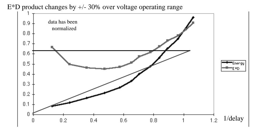
With modern technologies, max operating voltages is not very energy efficient
