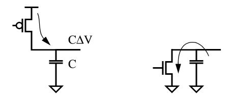
The average current that the 'capacitor' needs is just equal to the charge required to switch the capacitor time the number of times per second the capacitor switches. The latter term is just the frequency that the line is toggling at.
