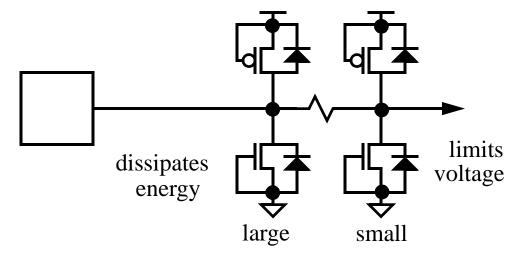
The diodes are the source/substrate diodes of the transistors. Near the pads you expect to have substrate currents. Need lots of well and substrate contacts. Even use guard rings - surround well with contact.
