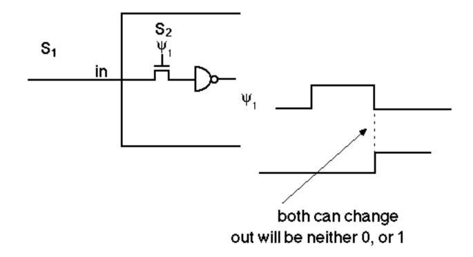
A simple dynamic latch could get an output that would be between 0 and 1.
