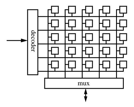
It has  $N^2$  elements and only 2N wires. It is an easy way to use 1M transistors. The layout is quite dense.
