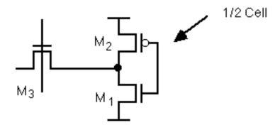
For the pull down M3 is passing a zero, so for it to overpower the pMOS it must be at least as wide (preferably 1.5x as wide). This gives a 2-3:1 current ratio between the nMOS and the pMOS.
