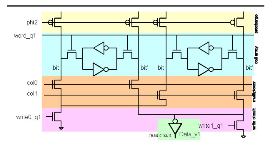
Should have a precharge on the output of the mux too, since otherwise the output will have a degraded high level.
