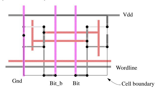
This layout is fairly dense, since the most of the contacts (bitline, Vdd, Gnd) are shared. Also the a clever cross-coupling method is used.
