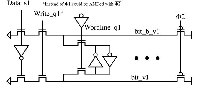
It is safer if the write drivers are complete tristate buffer (had a pullup device too) rather than just pulldowns. This will allow the driver to pull up a bitline that was partially discharged by the cell (if the wordline rises before the write signal)
