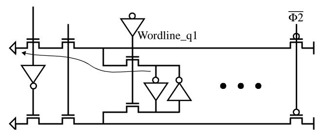
• If the pass device in the cell is 4:2, and the pMOS load is 3:4, then each nMOS in the driver must be at least 8:2. If the pMOS was 3:2, it would be hard to get the cell to write.
