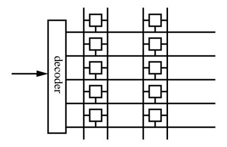
The decoder selects one cell on each set of bit lines. All the other wordlines are low, disconnecting those cells from the bitlines.
