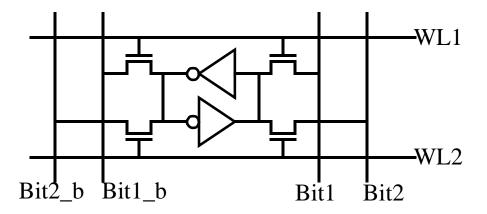
Shown in the figure is a true dual port cell. You can read or write on each port every cycle. Since it has more bitlines than the previous cell, it is much larger in area.
