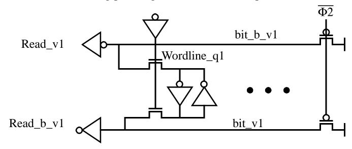
• Bitlines are like the outputs of normal precharge gates - \_v signals
