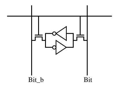
Read and write use the same port. There is one wordline and two bit lines. The bit lines carry the data. The cell is small since it has a small number of wires.
