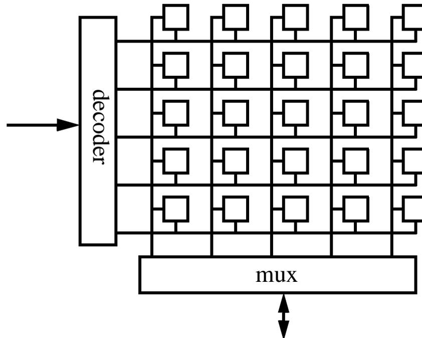
It has  $N^2$  elements and only  $2N$  wires. It is an easy way to use 1M transistors. The layout is quite dense. Most of the transistors in the million transistor chips are in memory arrays
