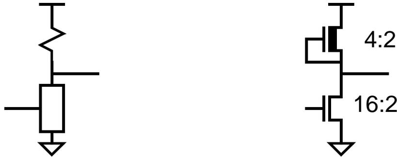
**Ratio Rule:** The resistance of the pulldown must be 4 times lower than the resistance of the pullup to guarantee a good low level (close to 0V).<sup>1</sup>
