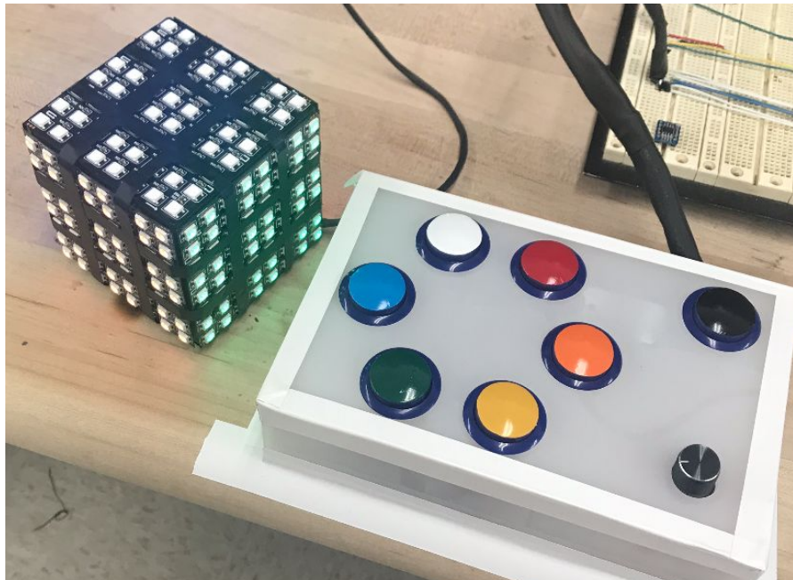
Figure 10: Our finished LED Rubik's Cube and user control panel.
