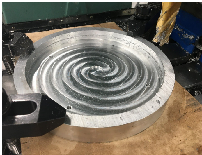
Machining flywheel interior
