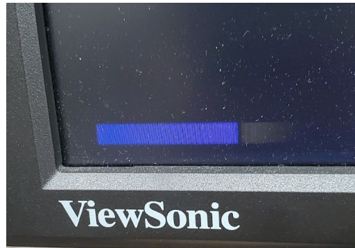
Figure 8. “Ghosting” of the blue line having a faint trail to the right
