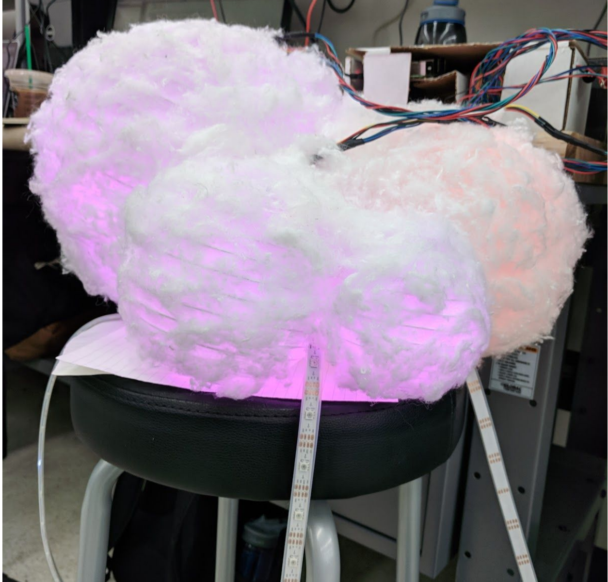
Figure 4: Completed Prototype. The cloud is displaying a sunset. The rain strands are not active. Hardware is visible in the upper right, protected from electrical shorts in a cardboard box.
