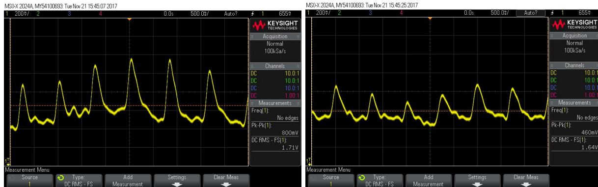
Figure 3: The oscilloscope outputs revealed that both DC offsets (left), and peak amplitude changed over time.
