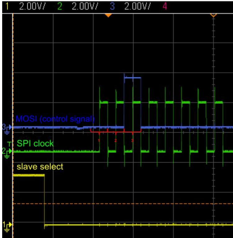
Figure 4: Example of the 17% (001) curtain control signal
