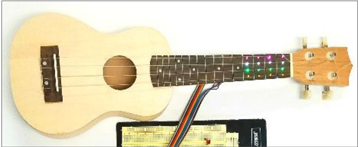
Figure 3: Full Ukulele Assembly. The small holes shown on the fifth fret have little to no impact on the user, while the first four frets show these holes allow adequate light to shine through, even in daylight and brightly lit rooms.
