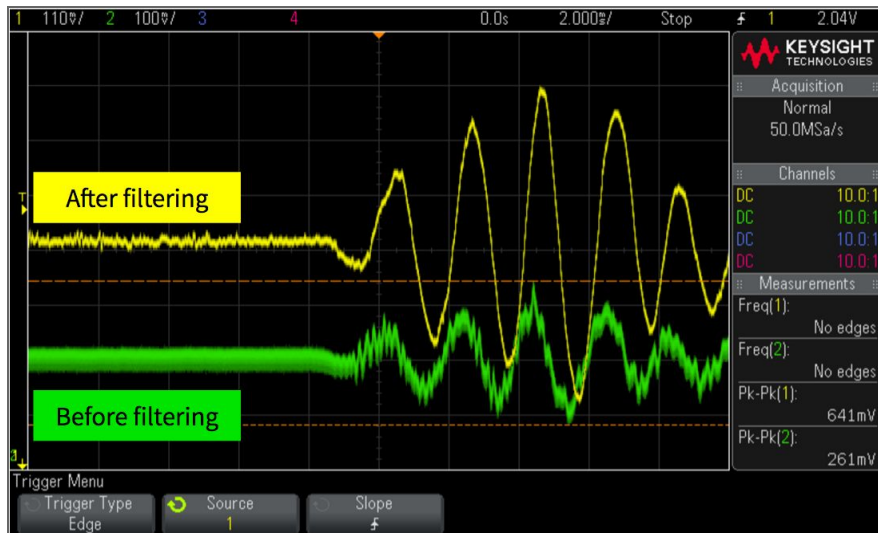
Figure 5: Sample Waveform. Oscilloscope capture of the contact microphone output when the A string of the ukulele is plucked. The green trace shows that before any filtering, the output exhibits a fair amount of high frequency noise and small peak-to-peak amplitude. After filtering, most of the high frequency noise has been removed and a gain has been applied.
