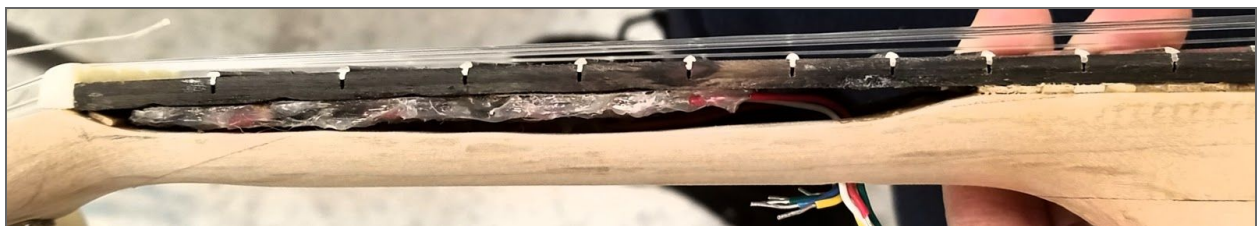
Figure 2: LED “sandwich.” The glue holding the LED array in place can be seen between the modified fretboard and neck.
