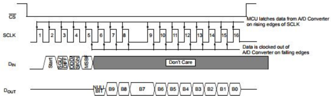
Figure 3. SPI Communication Protocol for MCP3002.
