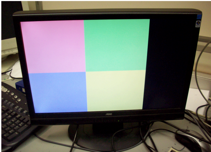
Figure 1: CRT Display Layout: The monitor is divided into four quadrants, each color corresponding to one button on the input pad. The color pattern is presented to the player by increasing the brightness of the appropriate quadrant.
