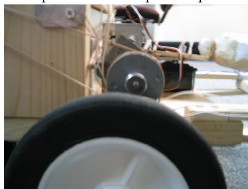
Figure 3: Motor drive system
