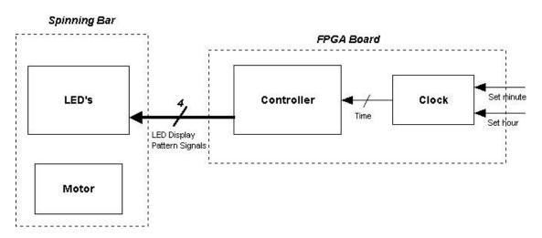
The spinning bar is a long strip of perfboard with the LEDs mounted on it. A motor is used to spin the bar at what we hoped would be a constant rate. The FPGA contains two blocks of logic. First, there is a clock which keeps track of time in hours, minutes, and seconds. There are lines into the clock to set the time, and lines out containing the current time.
