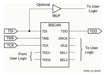
Figure 22: Boundary Scan Schematic Example
