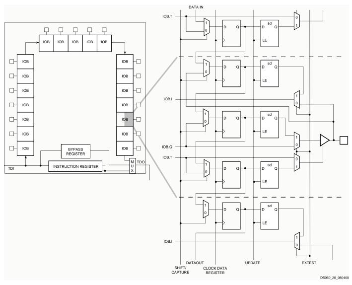
Figure 20: Spartan/XL Boundary Scan Logic
