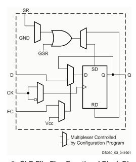
Figure 3: CLB Flip-Flop Functional Block Diagram
