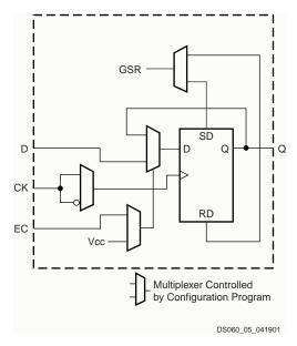
Figure 5: IOB Flip-Flop/Latch Functional Block
