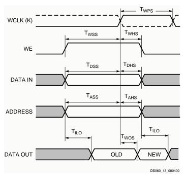
Figure 13: Data Write and Access Timing for RAM
