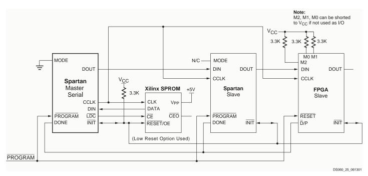
Figure 25: Master/Slave Serial Mode Circuit Diagram
