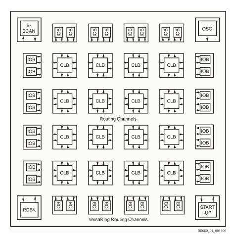
Figure 1: Basic FPGA Block Diagram
