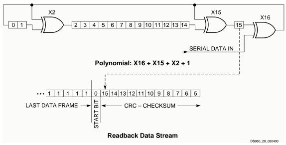
Figure 29: Circuit for Generating CRC-16
