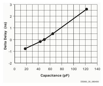
Figure 35: Delay Factor at Various Capacitive Loads
