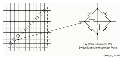
Figure 10: Programmable Switch Matrix
