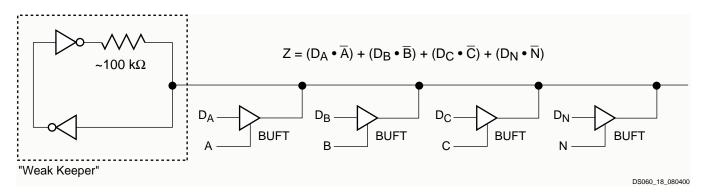
Figure 18: 3-state Buffers Implement a Multiplexer
