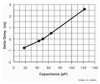
Figure 34: Delay Factor at Various Capacitive Loads
