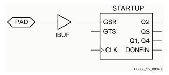
Figure 19: Schematic Symbols for Global Set/Reset
