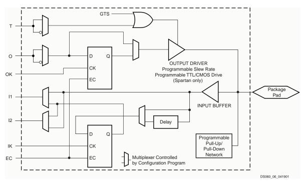
Figure 6: Simplified Spartan/XL IOB Block Diagram
