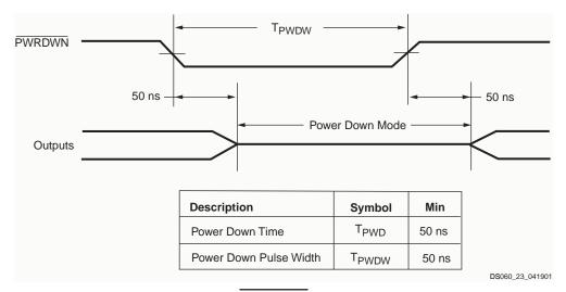
Figure 23: PWRDWN Pulse Timing
