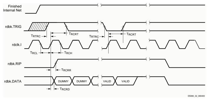
Figure 33: Spartan and Spartan-XL Readback Timing Diagram
