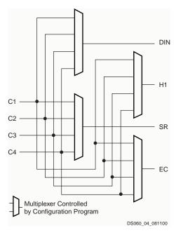
Figure 4: CLB Control Signal Interface
