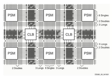
Figure 8: Spartan/XL CLB Routing Channels and Interface Block Diagram
