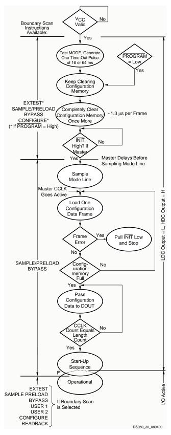
Figure 30: Power-up Configuration Sequence
