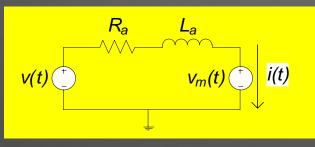
Shaft Angular velocity:  $\omega = v_m/K_e$ Torque: T=K<sub>t</sub>i(t)
