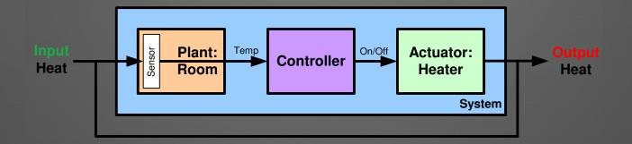
**Closed Loop Control is also called Feedback Control**
