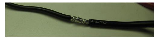
Once you're satisfied, clean up any stray wires with the cutters and wrap electrical tape around the junction. Then, do the same thing with the red wire from the battery pack and the black wire with the white stripe on the barrel jack leads. Remember that it is very important the two solder joints do not make contact or else power will be shorted to ground. You should end up with the following:
