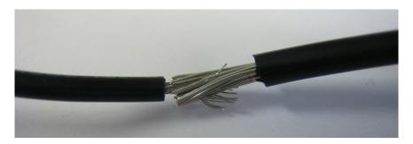
Heat the junction, and apply copious amounts of solder. Make sure that the solder is actually soaking into the connection, rather than just wetting the surface (if this isn't happening, keep heating the wires). You should also flip over the wires and solder the other side. You want to make a very strong electrical and mechanical connection.
