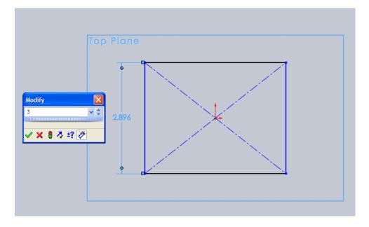
Now, repeat the process for the long side, making it 5.375" long. All the lines of the rectangle should now be black, and you should see "Fully Defined" in the status bar at the bottom of the screen. We're all done with the sketch, so click on *Exit Sketch* in the upper left corner of the Sketch tab. **Important:** Remember to **Exit Sketch** at the end of each feature you add!
