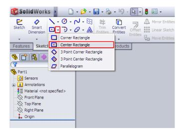
A set of planes should show up in the main window. Click on *Top Plane*. This means you'll be seeing the part from above. At this point, you should change perspective to make drawing more intuitive. There is a button on top of the main window that lets you select a perspective-this is the View Orientation button. Use it to shift into downward-looking viewpoint.
