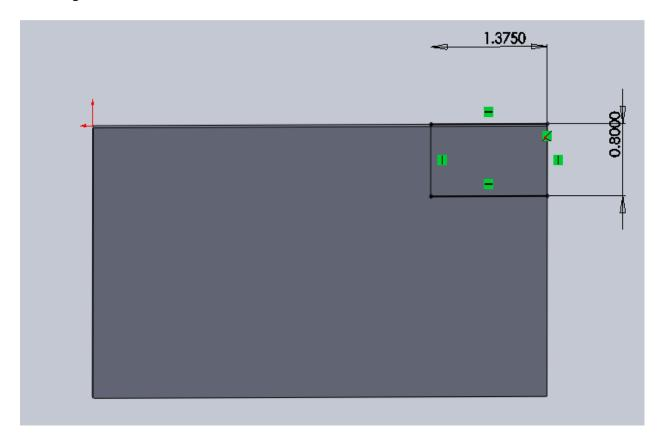
To save on effort, we will now mirror this rectangle along the long axis of the base. Select *Centerline* in the Sketch tab. This tool will be very useful for making symmetric parts.
