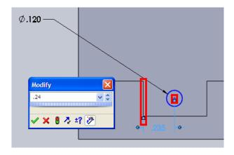
This sets the perpendicular distance from the edge to the center. You want this value to be 0.24". Similarly, set the distance between the circle's center and the bottom of the inset at 0.18". The final set of dimensions should look like the following:
