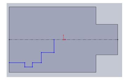
Be careful to keep that the lines stay either horizontal or vertical. Make sure that the line starts on the side of the base, and ends on the centerline. SolidWorks gives you visual cues (e.g. changing colors) to show when it's snapping points to other lines on the drawing.
