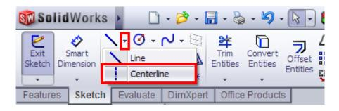
The centerline should connect the midpoints of the left and right sides of the base. Move the mouse along the left side of the base. When you are near the middle, an orange square should appear, indicating the midpoint of the line. Click on the square to start the centerline, move horizontally to the right side's midpoint, and click again to place a vertex. Press Esc once or Enter twice to complete the line.
