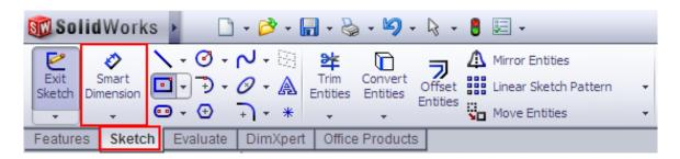
Click on the rectangle's left side, move the cursor a bit to the left, and click again to place the dimension on the sketch. At this point, a window should pop up allow you to set the dimension. We want the rectangle to be 3" by 5.375", so enter 3 in the window and click the check box.
