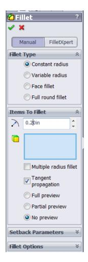
The top icon under "items to fillet" is asking for a radius to determine how much rounding to do. Enter 0.2". Now, the blue box wants edges to fillet. You can enter these by holding your mouse over the area you want until you see the element highlighted in orange:
