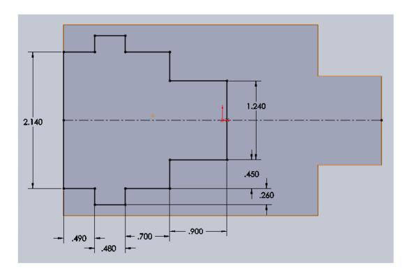
Now, exit the sketch. Set the extrusion's end condition to "Blind", and pick a depth of 0.1". This will cut part way through the body. Complete the extrusion, and look over your work.
