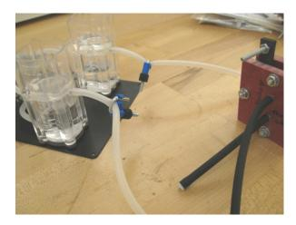
Note: Mark the side hooked up to the hydrogen as the anode using a Sharpie. This will now always be the side hooked up to the hydrogen for future setups.
