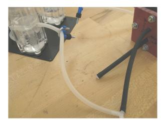
If there is a leak (seen by a sharply declining hydrogen level in the electrolyzer), this means an inlet or outlet tube (port) is not fully sealed in the endplate. Either add more silicone adhesive or, if there are large gaps, remove the tube and reseal it.
