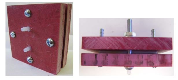
Add the tubing stoppers on three of the four gas ports. Hook the remaining port up to the hydrogen side of the electrolyzer. Unplug the electrolyzer, so that the generated hydrogen is a fixed volume trapped in the tank.
