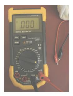
Third, set up the circuit to measure the fuel cell's output current. You will be doing this with a different multimeter, setting it to be used as an ammeter. Put the variable resistor and ammeter in series with the fuel cell. This way you can vary the load on the fuel cell and measure how the current and voltage vary.
