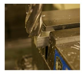
13. Move the table in the y-direction so you are no longer above your part. Engage the fine adjust wheel and then unlock the quill. You can use this wheel to move the quill (and by extension the endmill) in the z-direction. Lower the endmill to -0.050" in the z-direction (also known as "50 thou", short for "50 thousandths" since one thousandth is 0.001"). Make a cut by moving the y-direction through the material, just like step 6.
