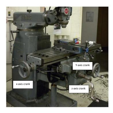
6. Start with the material behind the endmill. Once the endmill is spinning, apply cutting oil with the brush and gradually move it forward to face the first end. The slower you move, the smoother the cut.
