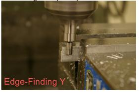
Since the edge finder has a part diameter of 0.2", you must configure the DRO to correspond to 0.1" below the edge of your piece. Program -0.1" into the y-dimension. By setting the DRO, you are, in a sense, superimposing a coordinate frame onto your part.
