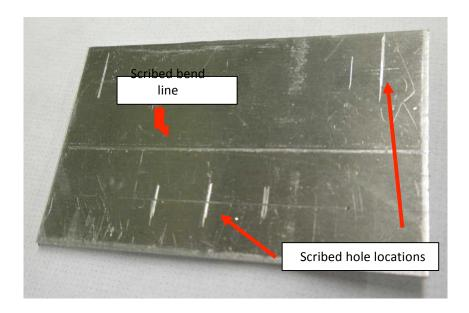
5. Use a hammer and center punchGot it. to create a small divot at each desired hole location. This will be used to properly position the hole punch.
