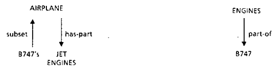
Fig. 4(a). Semantic nets showing that B747s have jet engines (After Barr and Davidson, p. 148 [16])
